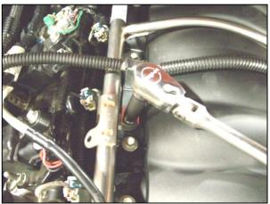
10. Measure 25mm (1 inch) inward from the edge of the bracket and mark the bracket with a line.
