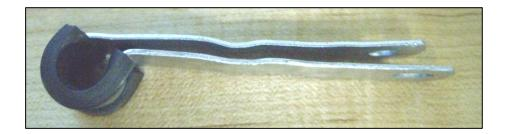
12. Re-bend the bracket at the location that was marked in step 9.
