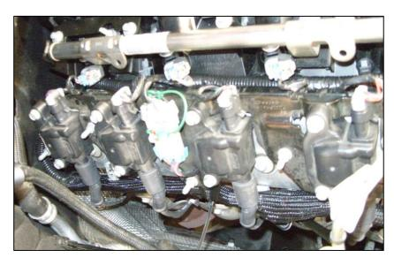
19. Remove and discard the three (3) bolts retaining the ignition coils in the location noted in the image below.
