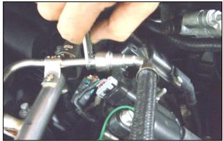
NOTE: BE SURE THE FUEL RAIL IS FREE FROM DRIPS TO PREVENT FUEL FROM CONTACTING THE SILVER SLP PAINT. THE SILVER SLP PAINT IS NOT SOLVENT RESISTANT.
