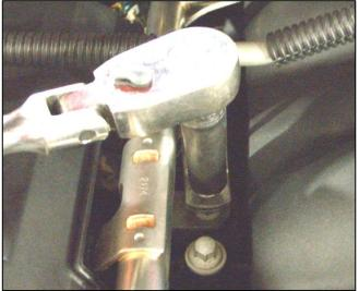
26. Position the VMV line over the newly installed coil cover and connect it to the VMV solenoid. Note: For SLP supercharged applications, the VMV line will be routed underneath the coil cover since the valve was relocated during supercharger installation.
