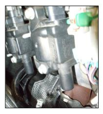
17. Re-route the wiring harness noted in steps 13 & 14 so it is just below the coil bracket and zip tie it in place as shown in the image below. Cut the tail of the zip tie so it is flush with its retainer.
