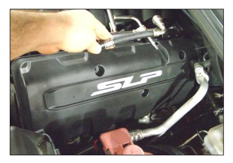
32. Install the three (3) bolts (PN F161814 for coil style A, PN F161813 for coil style B) included in the hardware kit (PN COILKIT-HWKA-AA) into the locations identified in the image below. Torque the three (3) bolts to10 Nm (89 in/lbs).
