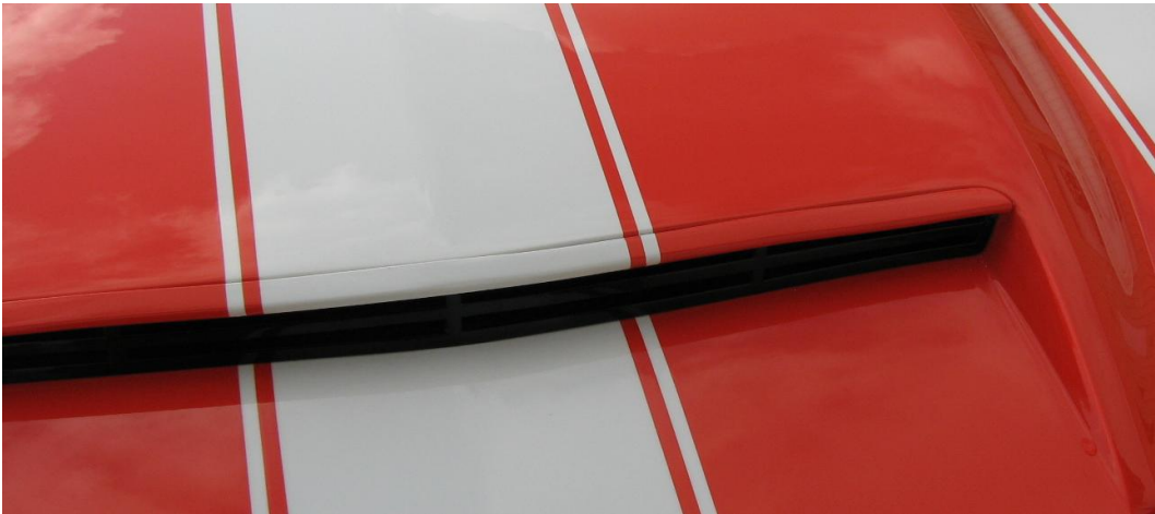
Figure 4: Finished hood grille installation
