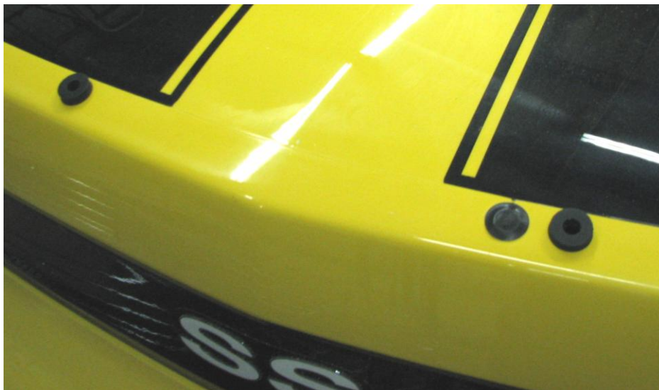
Figure 6: Rubber washer and sheet metal plug placement
