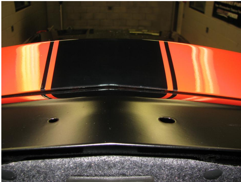
Figure 1: Slight overhang of rear spoiler (view with deck lid open)
