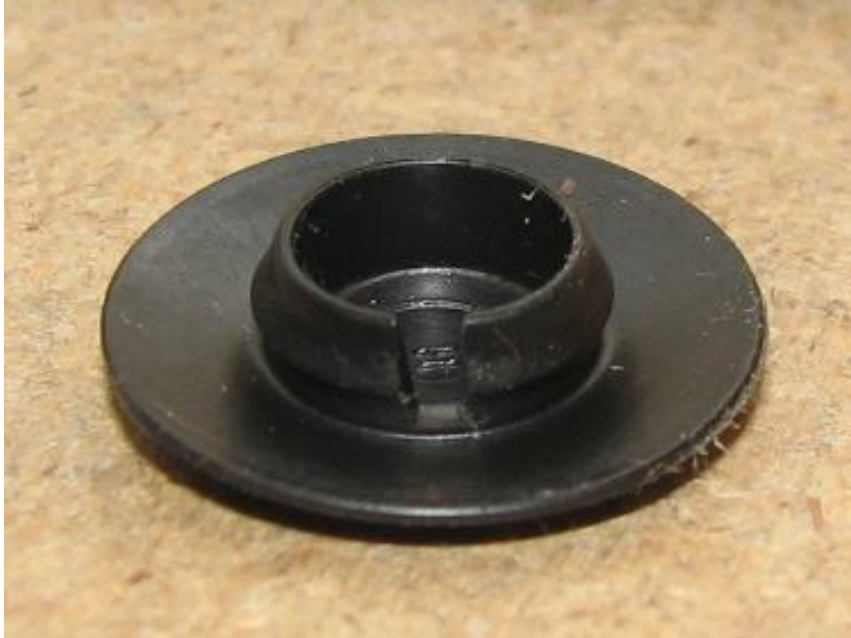
Figure 5: Slot cut into sheet metal plug
