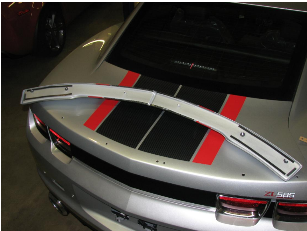
Figure 3: Rubber strips and foam washers applied
