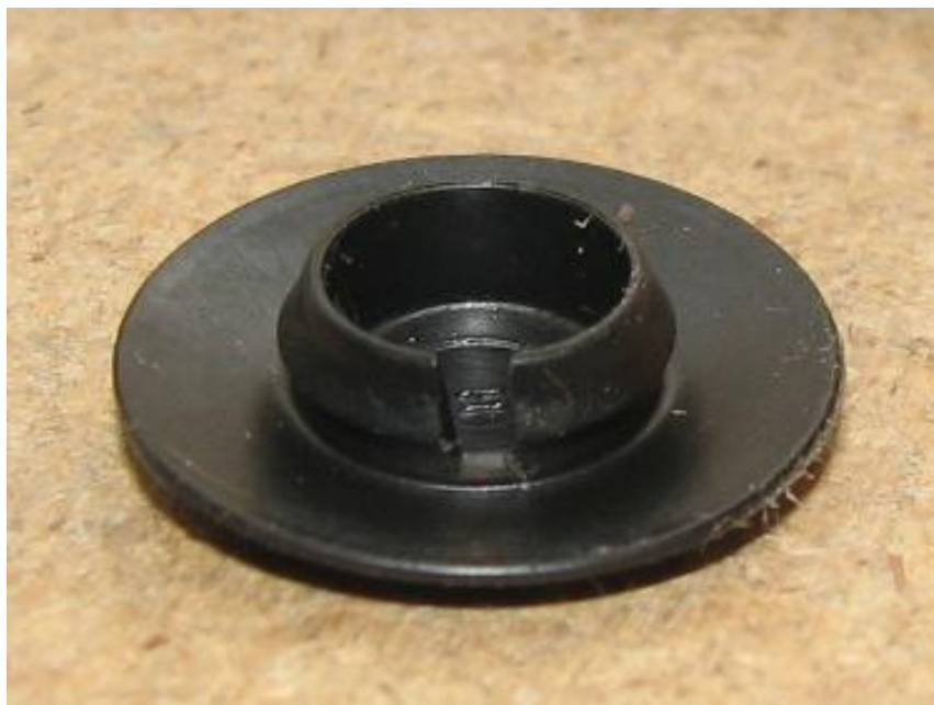
Slot cut into sheet metal plug
