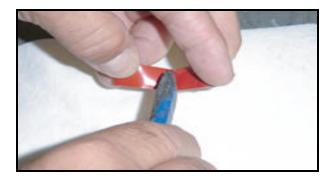
**5.** Remove the red tape backer. Insert light into part as shown below. Apply 35lbs of pressure to taped areas.
