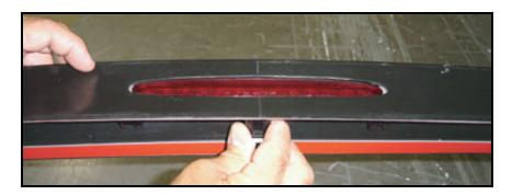
**2.** Clean tail light and rear spoiler at bond Zone with alcohol and water solution (50/50mix).
