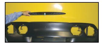
2. Remove middle tail light housing Unhook the break light connection.
