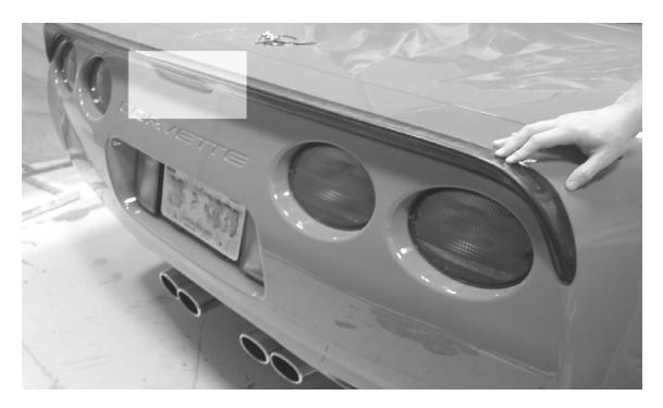
**Step 6:** Starting from the center of the wing peel red tape backing from lower tape surface and stick to the car working your way toward the ends of the wing.
