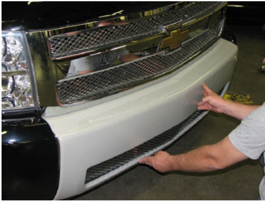
Photo 2: SLP Overlay Installed
