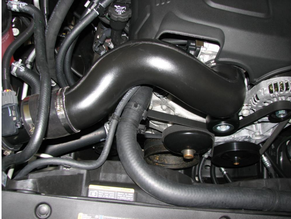
Figure 6: Installed intake tube with adaptor hose
