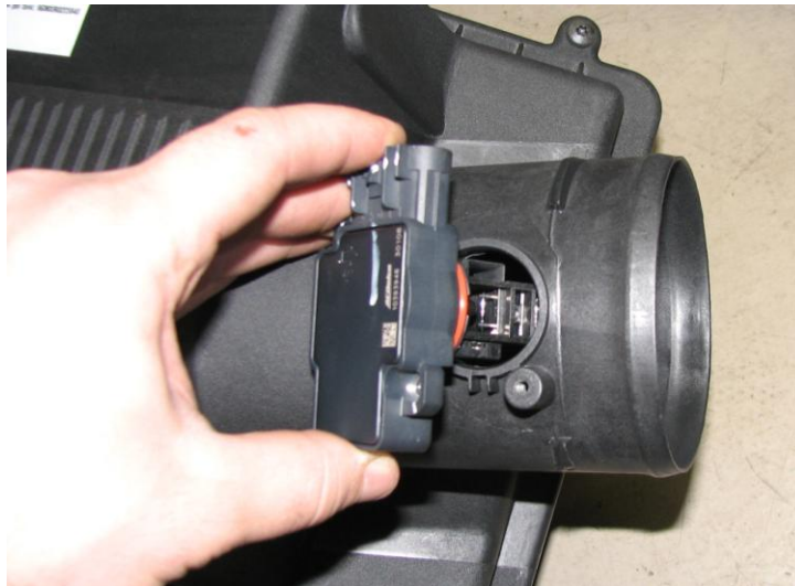
Figure 2: Removal of factory MAF from airbox
