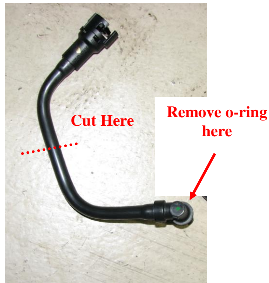
Figure 7: PCV hose cut location
