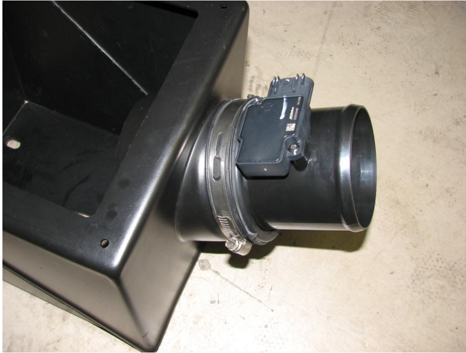
Figure 3: MAF and airbox adaptor placed onto airbox
