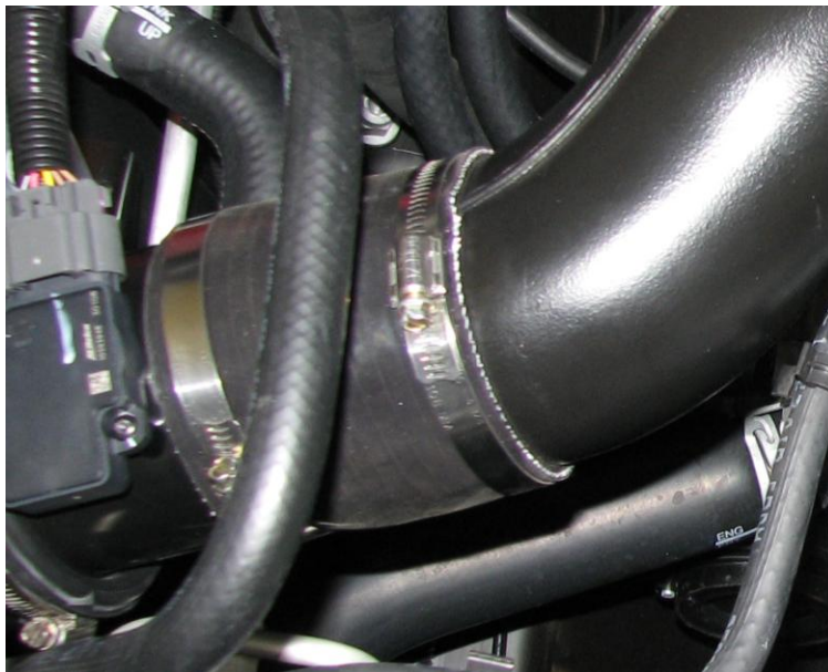
Figure 5: Rubber inlet adaptor installed with clamps
