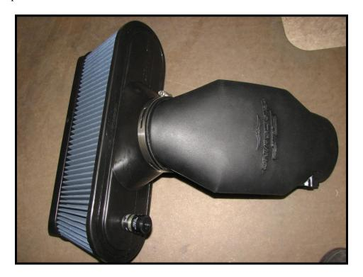
10. Next, remove the STOCK MAF from the STOCK airbox assembly and install the MAF into the SLP Blackwing Airhorn using the <u>SUPPLIED</u> torx screws. Make sure the square rubber seal remains on the MAF when removing and installing. **Only tighten** the MAF screws until the backside of the MAF mounting surfaces touches the SLP black mounting standoffs then stop. Make sure that the flow arrow is facing the outlet of the new Airbridge. The MAF can only install one way.
