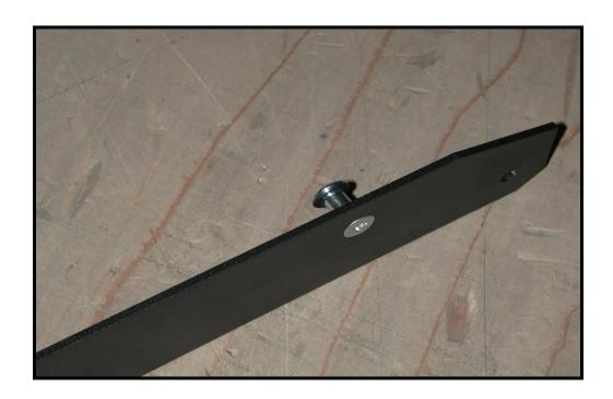
3. Next install the supplied frame nuts using the supplied 3M adhesive. See photo below of placement of frame nuts. Use the 3M adhesive on the backside of the frame nut flanges. Insert the frame nut into the frame hex hole and hold in place for 45 seconds each. Let dry for 15 minutes then proceed to step 4 below. See photos below for mounting locations of frame nuts.
