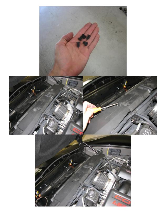
7. Next install the rubber grommets supplied into the SLP Blackwing filter as shown in the photo on the next page.
