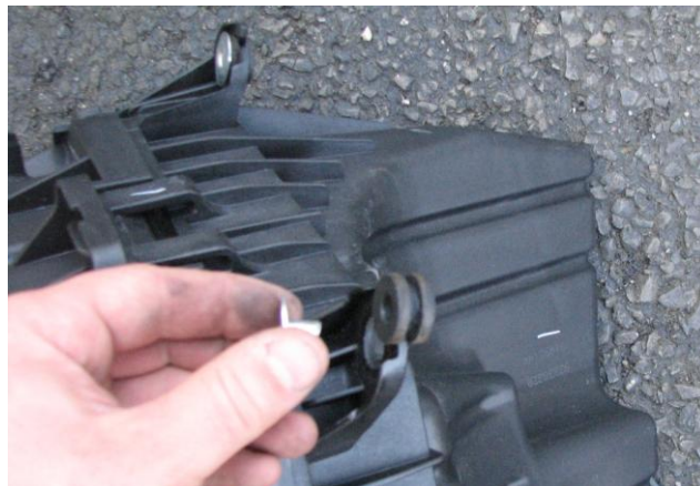
Figure 12: Removal of rubber isolator
