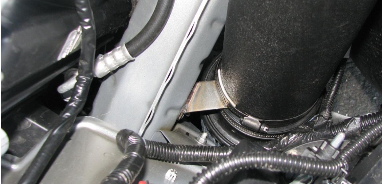
Figure 24: Tightening of worm drive clamp over bracket.
