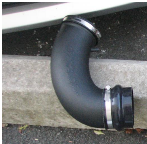
Figure 21: Upper intake tube with bellows and TB adaptor installed
