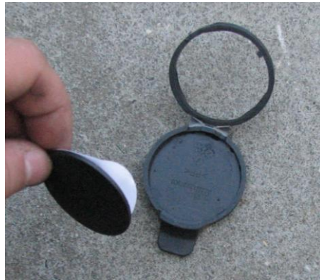
Figure 9: Rubber seal in washer cap
