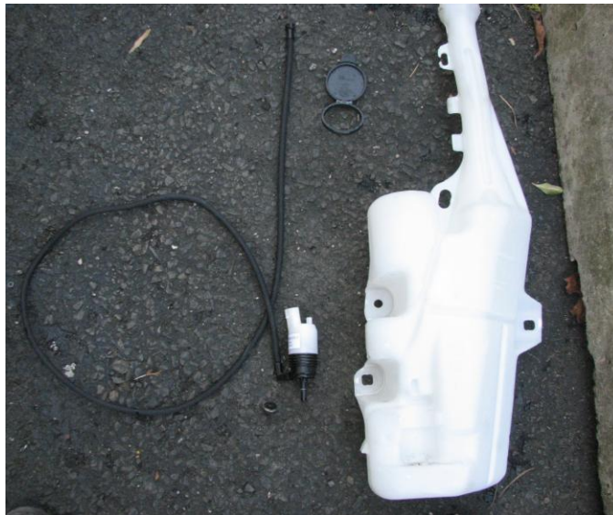
Figure 6: Factory washer bottle with components removed
