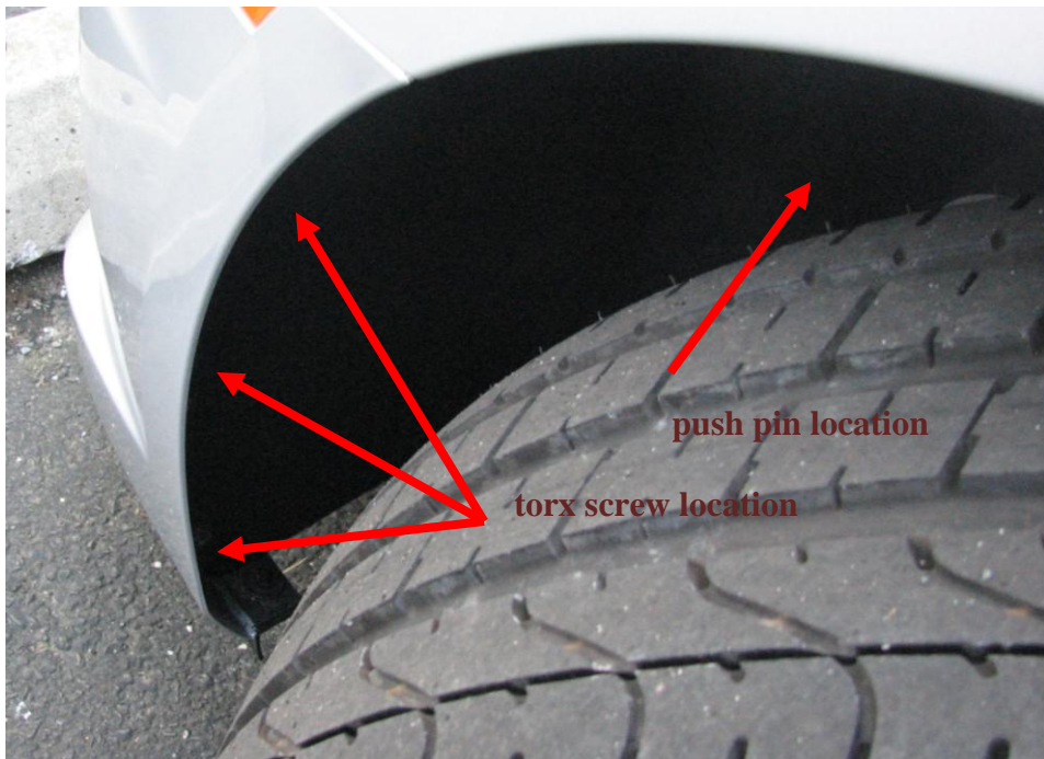
Figure 2: Screw removal in fender well
