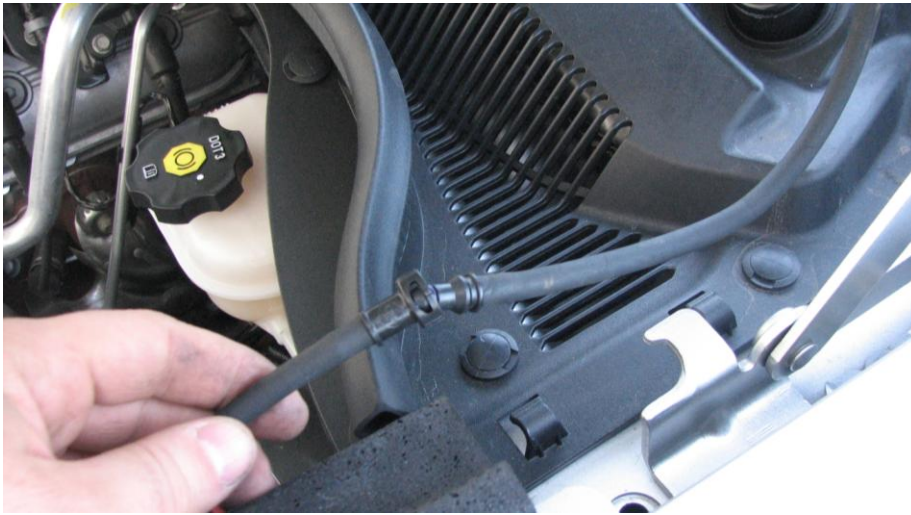
Figure 4: Disconnecting the windshield washer line
