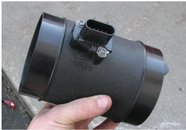
Figure 1: Factory MAF installed into SLP MAF tube
