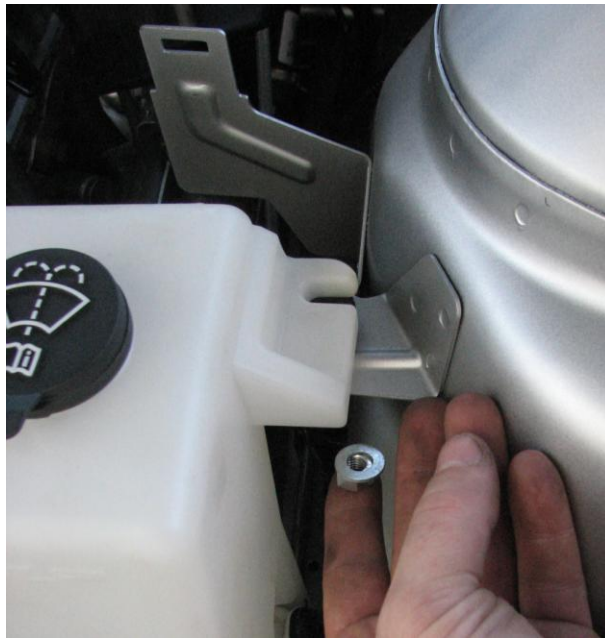
Figure 15: Tip for easily threading the nut onto the bolt
