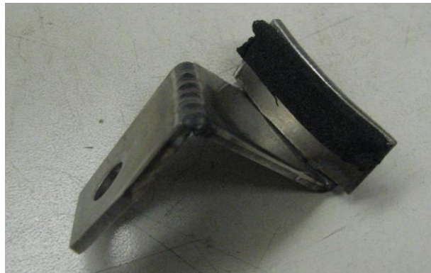
Figure 16: Foam tape on inside of bracket
