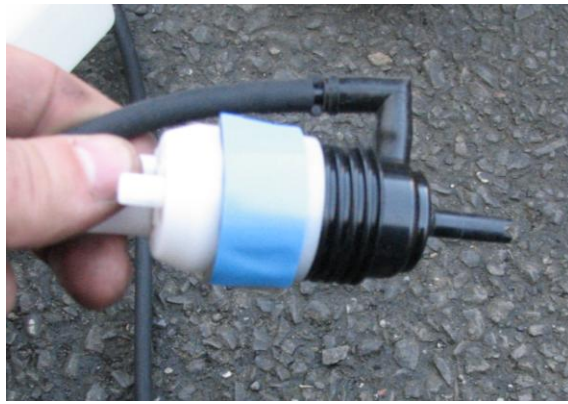
Figure 8: Tape applied to washer motor
