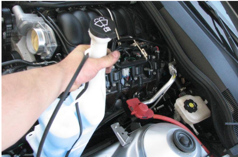
Figure 5: Removal of windshield washer bottle from vehicle
