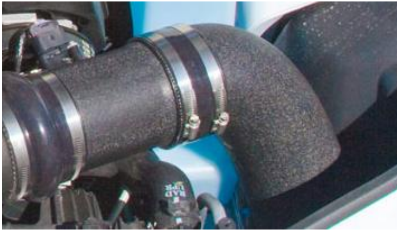
Figure 20: Location of clamps on outside of bellows with worm drive screw facing forward
