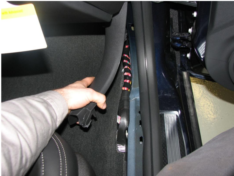
Photo 11: P-side kick panel removal
