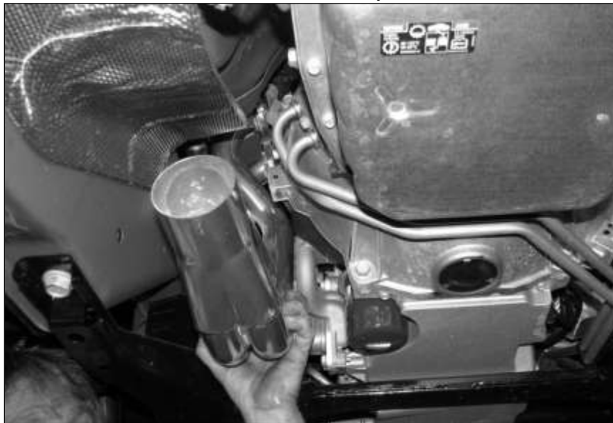
Figure 3: Insertion of driver's side header
