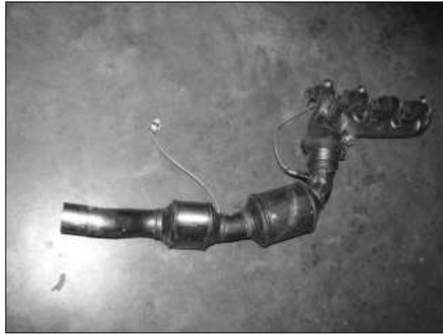
Figure 1: Passenger side manifold removed
