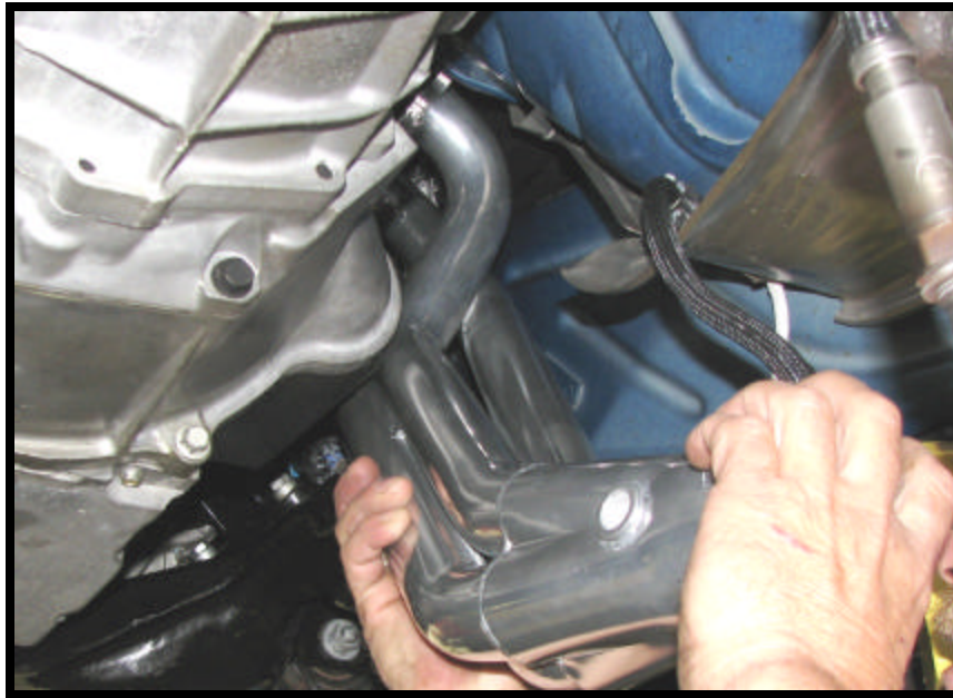
Photo 2: Installation of the Passengers Side Header
