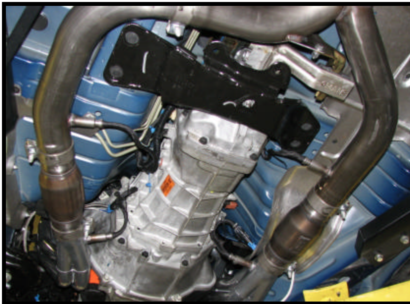
Photo 3: SLP Y-pipe Installed
