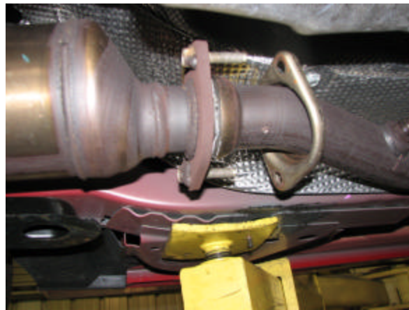
Figure 2: Removal of ball flange nuts
