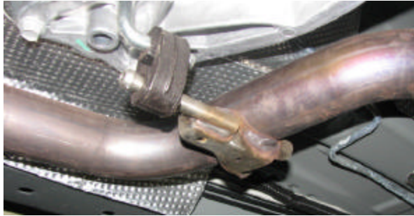
Figure 3: Front rubber exhaust hanger removal
