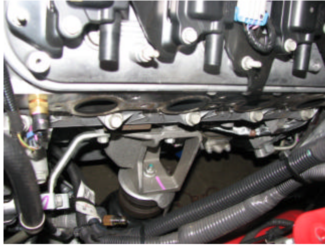
Figure 5: Driver side manifold removed
