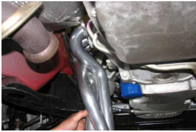
Figure 7: Insertion of driver's side header
