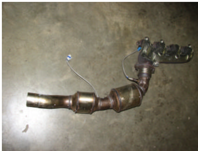
Figure 1: Passenger side manifold removed
