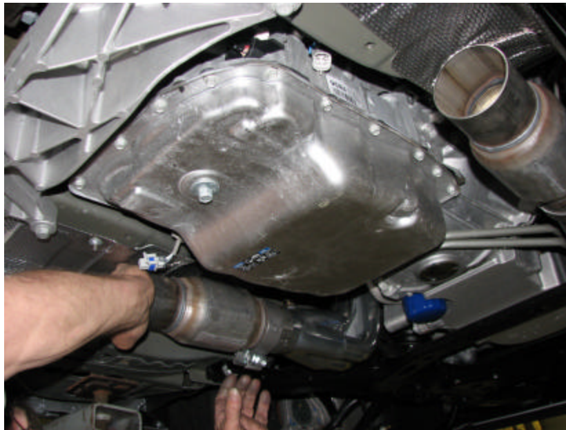
Figure 4: CATs installed onto headers
