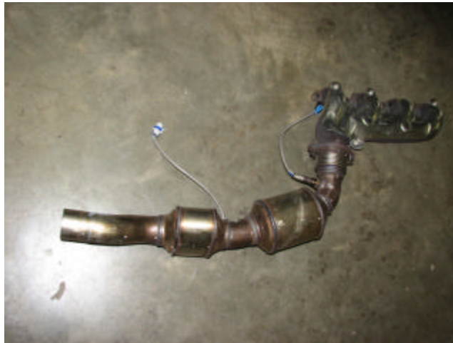
Figure 1: Passenger side manifold removed
