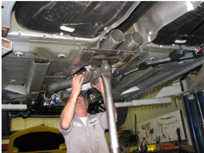
Figure 7: Installation of X-Pipe assembly
