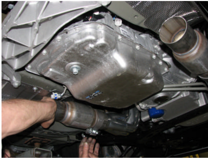
Figure 4: CATs installed onto headers
