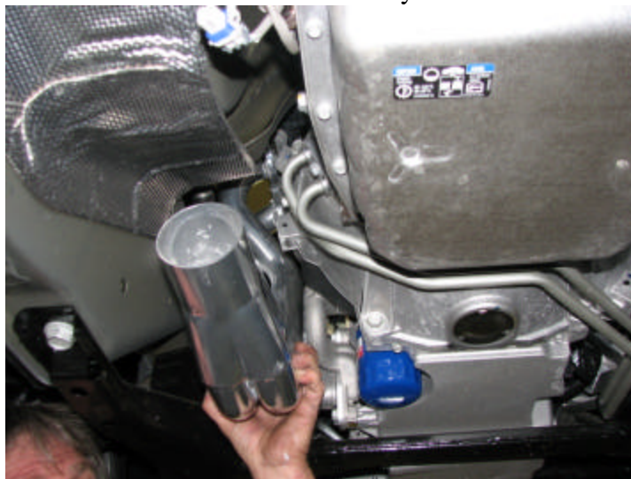
Figure 2: Insertion of driver's side header
