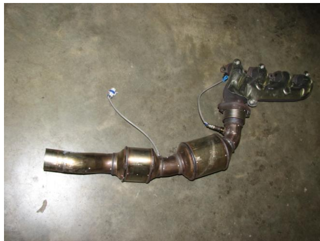
Figure 2: Passenger side manifold removed
