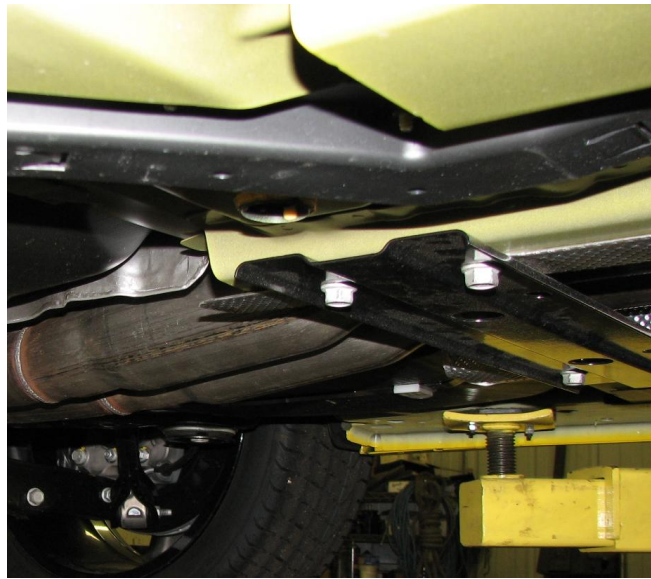
Figure 1: Removal of center support bar
