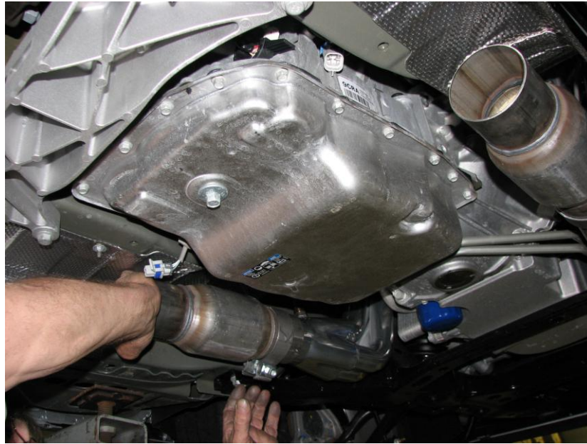
Figure 5: CATs installed onto headers
