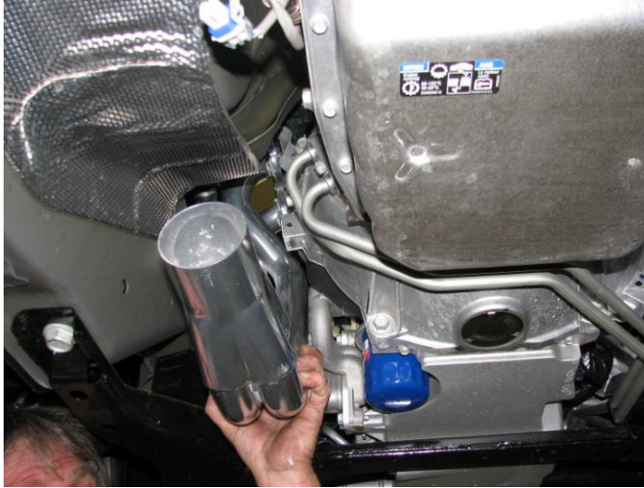
Figure 3: Insertion of driver's side header
