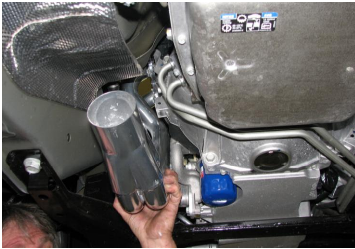
Figure 2: Insertion of driver's side header
