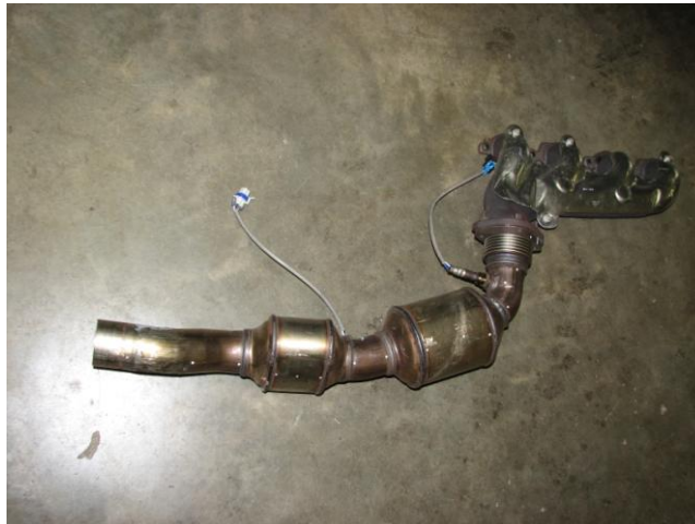
Figure 1: Passenger side manifold removed
