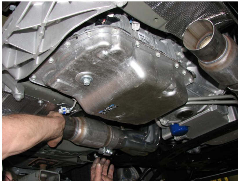
Figure 3: CATs (or CAT replacements) installed onto headers
