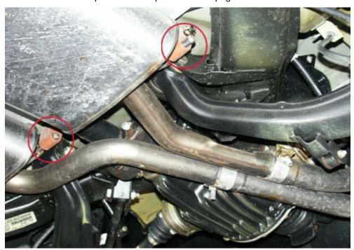
7. Next remove the four bolts that attach the stock X-Pipe to the catalytic converter pipes. Retain the four bolts as you will re-use them to install the SLP exhaust system. See photo below.
