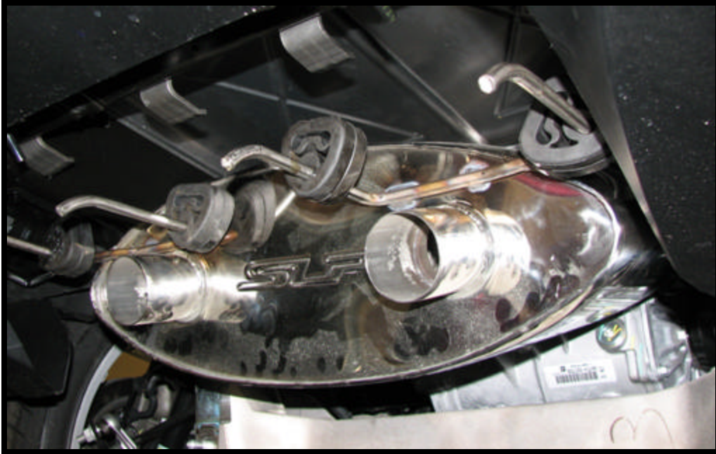
Photo 5: Muffler Installed on Over-axle Pipes
