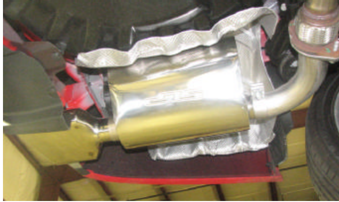
7 Figure 3: Installation of driver side section
