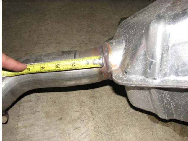
Figure 1: 1.75” from weld on rear muffler
