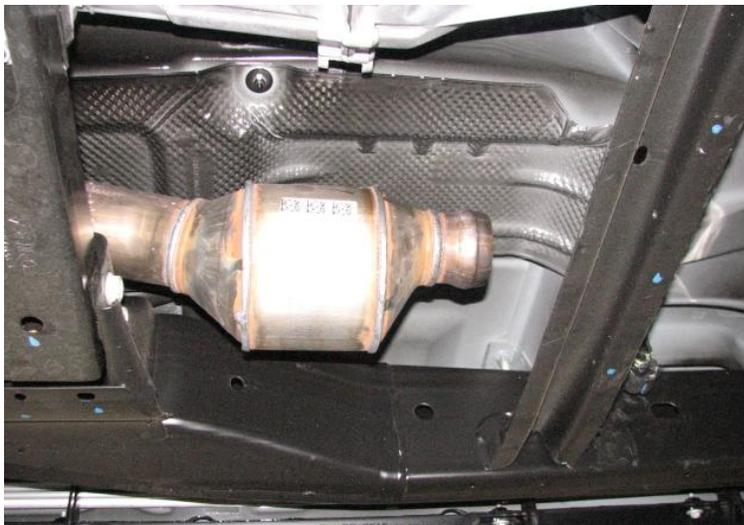
**Figure 2: Removal of factory flex joint**
