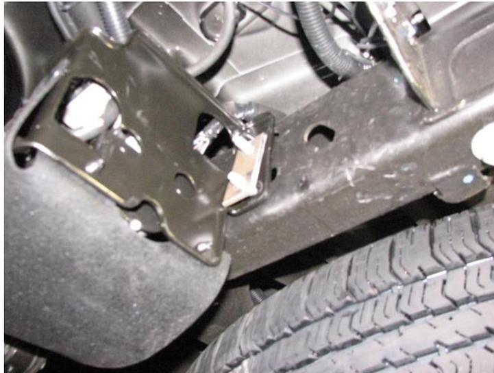
**Figure 4: Hanger spacer being placed onto the bolts in frame**
