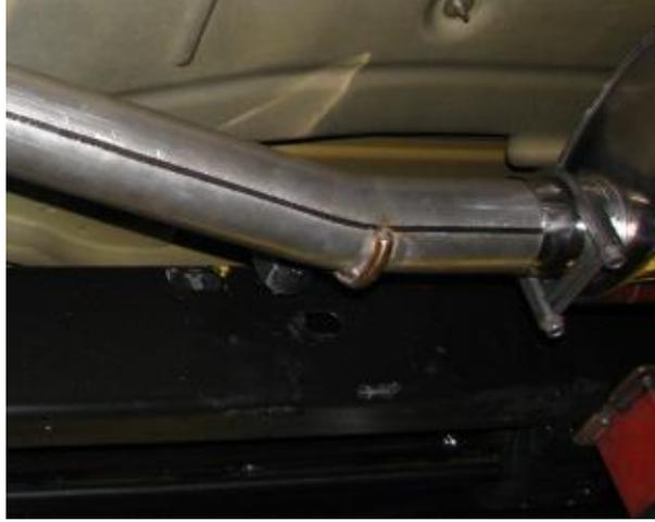
**Figure 7: Intermediate pipe attachment to muffler**
