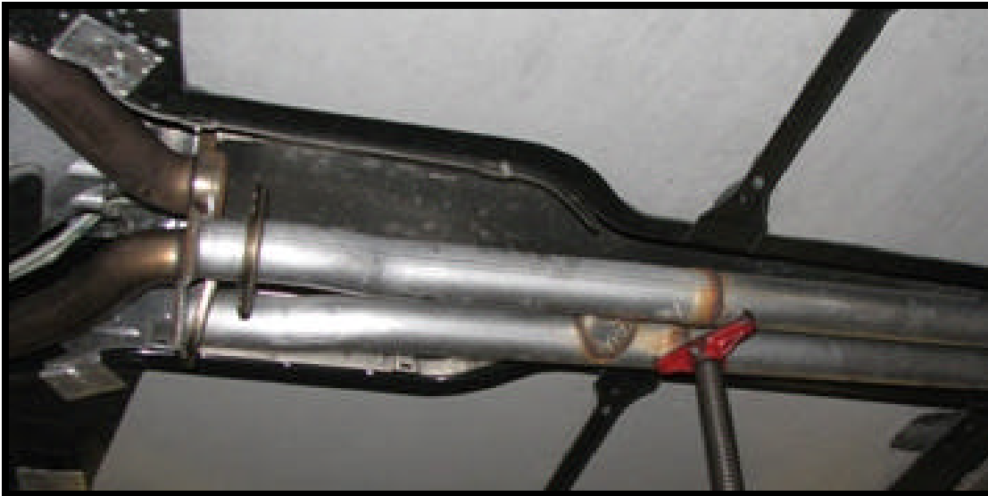
Photo 1: Factory H-Pipe Removal
