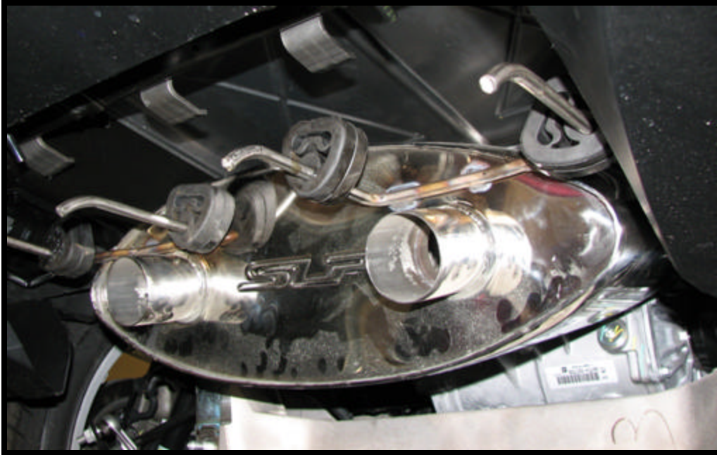
Photo 5: Muffler Installed on Over-axle Pipes
