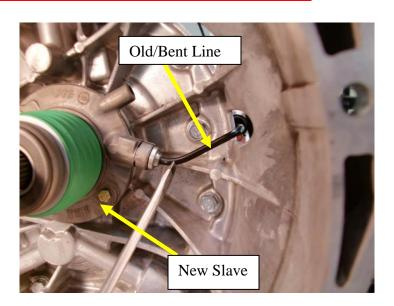
5. Going back and forth using the old slave on the bench. Fit the line the rest of the way as shown below. You will need to straighten the line as shown in two places below.
