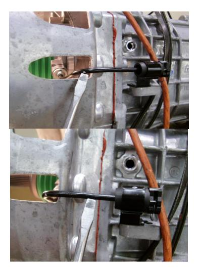
6. When complete make sure line is bent correctly so that no stress is on the orings or line when bracket is mounted.
