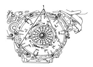
5. Ensure all three dowel pins (1) are visibly seated through the clutch cover
