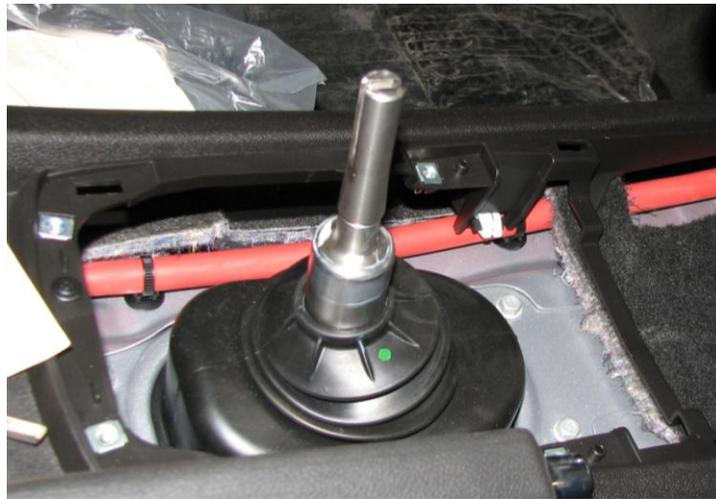
**Figure 10: Upper protective boot in place**
