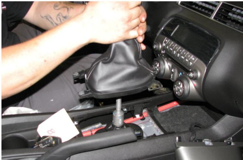
**Figure 3: Removal of shift knob**
