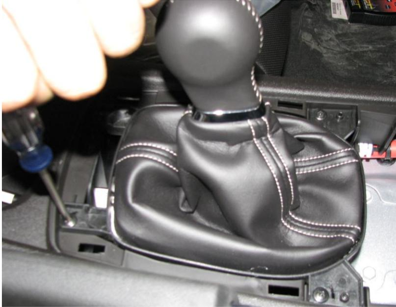
**Figure 2: Removal of 4 screws holding down shifter boot**
