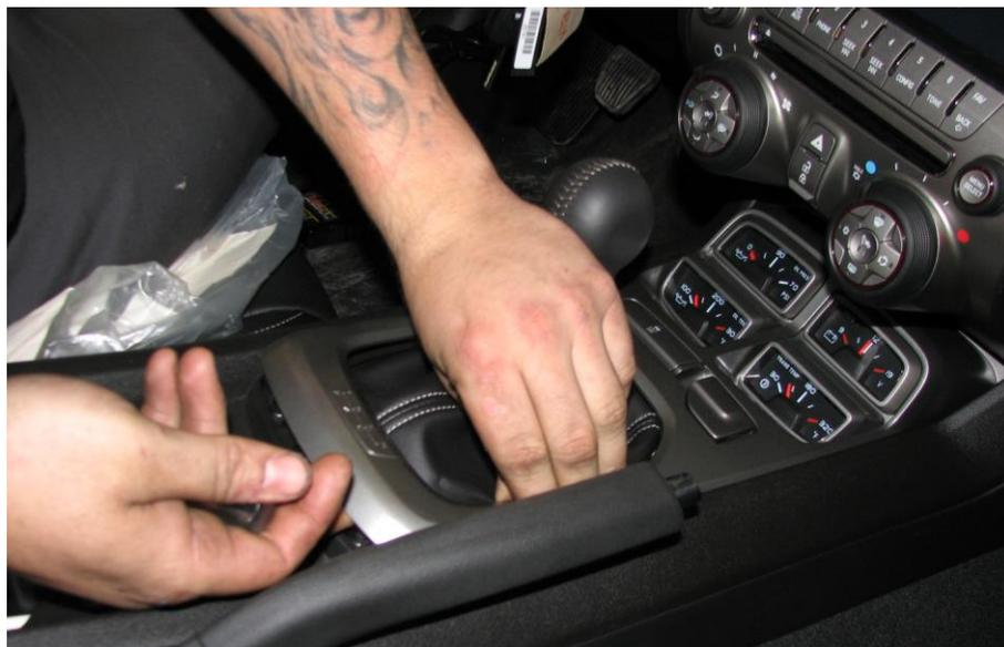
**Figure 1: Removal of shifter trim**
