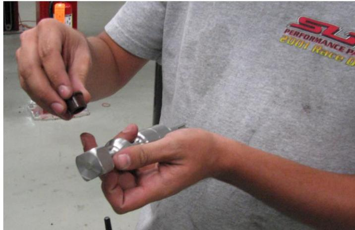
**Figure 7: K-Prene Bushing installation**
