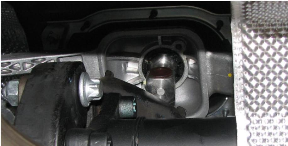
**Figure 9: Installation of bushing endcap and bolts**
