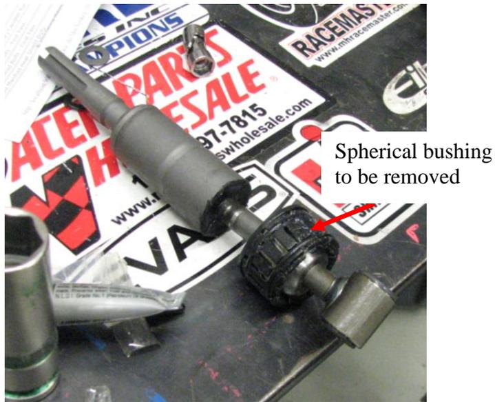
**Figure 6. Spherical bushing and seal to be removed**
