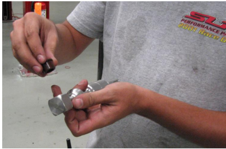
Figure 7: K-Prene Bushing installation
