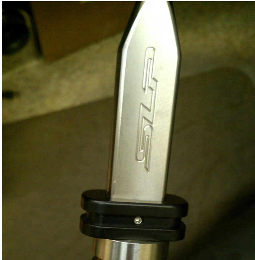
Figure 11: Use set screw to fasten trim ring to shifter
