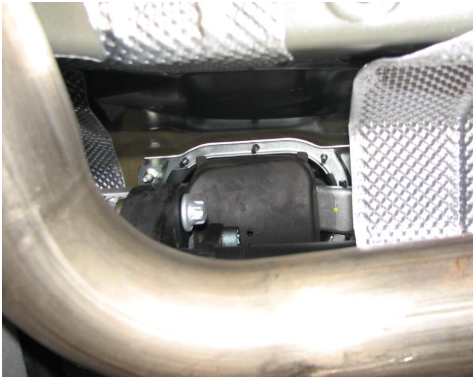
Figure 4: Black boot to be pushed aside
