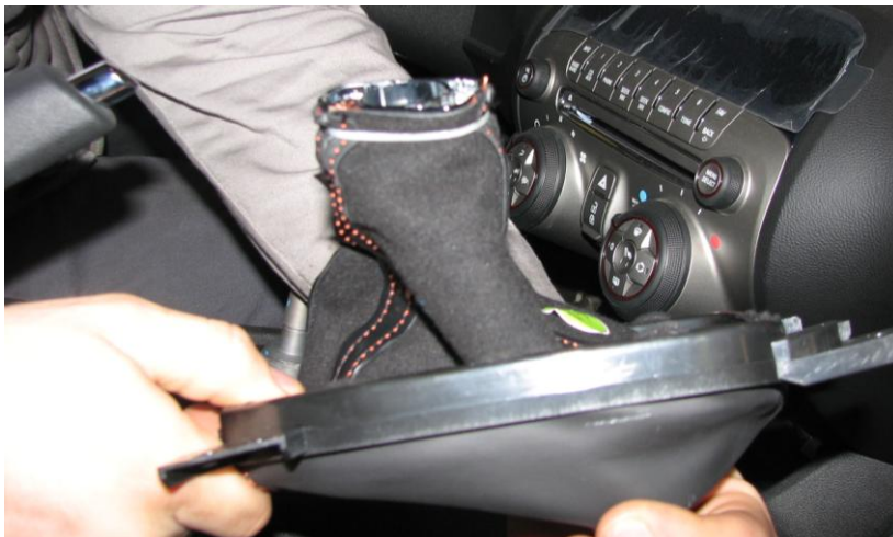
Figure 12: Turning the shift boot inside out to remove zip tie
