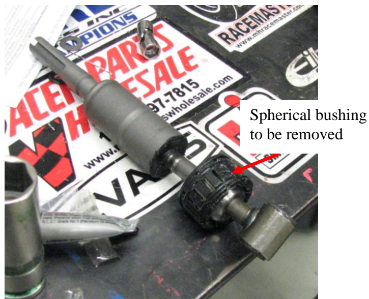
Figure 6. Spherical bushing and seal to be removed
