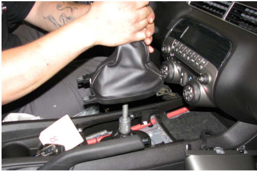
Figure 3: Removal of shift knob
