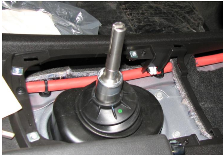
Figure 10: Upper protective boot in place
