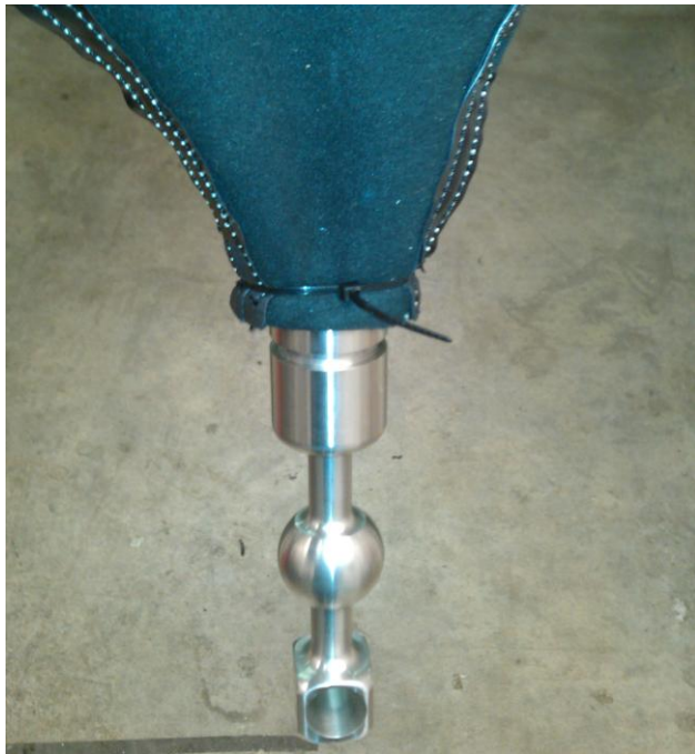
Figure 13: Attachment of the shifter boot to the shifter trim ring
