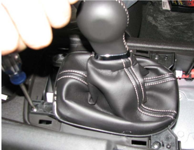
Figure 2: Removal of 4 screws holding down shifter boot
