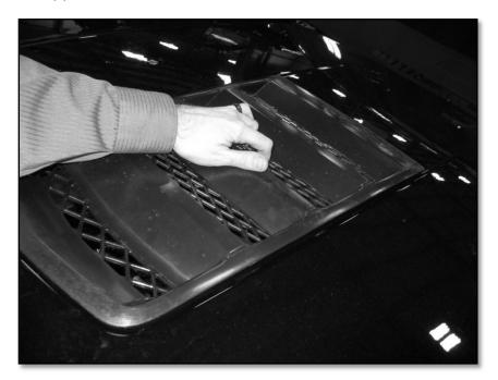
6. Loosely install the six(6) 10mm nuts onto the upper heat extractor. Then check the positioning of the extractor before final tightening. Do not over tighten, you can crack the extractor.
