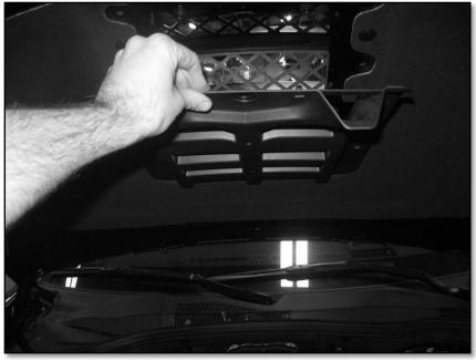
4. Remove the two(2) plastic clips holding the hood blanket to the hood.
