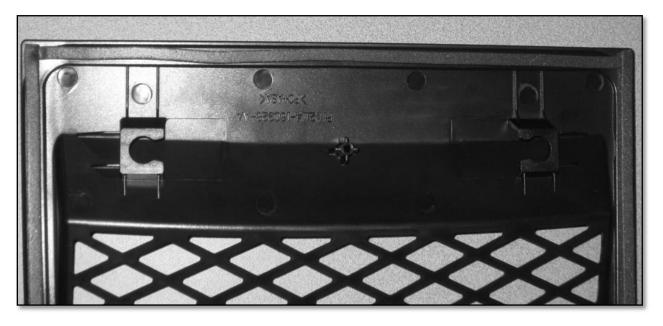
4. Install the six(6) M6 bolts from the factory heat extractor into the new upper heat extractor.
