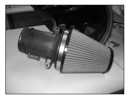
4. Install the mass air tube and filter into the airbox and tighten the two provided M8 bolts using a 10mm socket.
