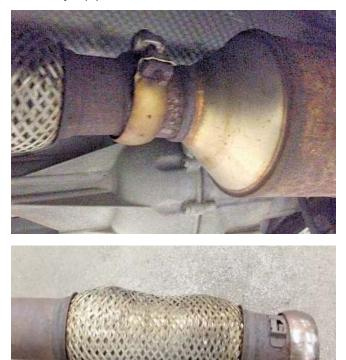
2. Remove the factory exhaust by disconnecting each exhaust hanger from the exhaust system.
