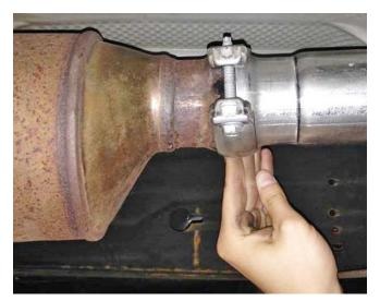
Install one (1) 3" clamp (P/N: 10-0439) over the outlet of the over-axle pipe and install the tip (P/N: 310305787) onto the outlet end of the overaxle pipe. Position and orient the tip to the desired location. Position the clamp on the joint and tighten to 30 Nm.
