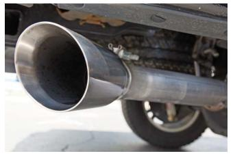
Before starting the vehicle, make sure to check all wires, hoses, brake lines, body parts, tires and any other components for safe clearance from the exhaust system.
