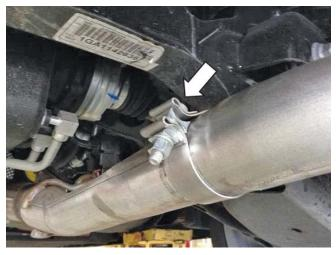
6. Slide one (1) of the 3" band clamps (P/N 10-0439) over the end of the LH and one (1) over the RH pipes.
