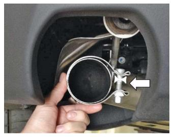
7. Carefully install one (1) tip (P/N 310305787) over each of the ends of the pipes. Slide the band clamps over the joints and align tips for the desired fit with the rear valance. Torque band clamp 15 mm bolts to 30 Nm. If adjustments are necessary, loosen the band clamp bolts, make your adjustments and re-torque the clamp bolts.
