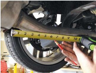
2. Cut the LH and RH exhaust pipes at the locations marked in step 1 using a suitable cutting tool.
