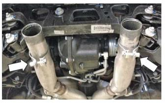
4. Insert the RH pipe (P/N 5-62 V8) or (P/N 5-65 V6/I4) over the RH under axle pipe and reattach the rear hanger to the frame using the original fasteners. Repeat the same procedure for the LH pipe (P/N 5-61 V8) or (P/N 5-64 V6/I4). Torque the hanger fasteners to 20 Nm.
