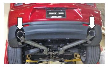
Before starting the vehicle, make sure to check all wires, hoses, brake lines, body parts, tires, and any other components for safe clearance from the exhaust system.
