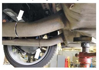
3. While supporting the muffler, detach the rubber hanger bushings closest to the axle from the hanger brackets on each side of the muffler.
