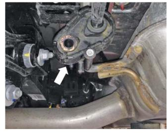
4. Unbolt the two (2) rear hangers from the frame located behind the rear bumper, and remove the hangers from the vehicle.
