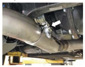
Align the front of each pipe to the installation depth, previously marked. Slide the band clamps over the joints and position as shown. Torque the band clamp 15 mm bolts to 30 Nm.
