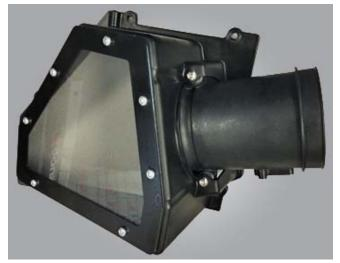
2. Install the air filter (997-484-BLK) with the metal tab pointing downwards. Tighten the clamp to 3 Nm.
