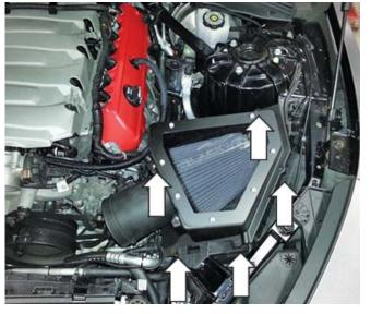
Install the clamps (R07130028-13-AA) and (R07130015-13-AA) from Hardware Kit A onto the clean air tube (2116-9B660). Install the larger diameter clamp (CT-32) onto the MAF tube side. Install the assembly on the throttle body and clean air tube. Torque to 3 Nm.
