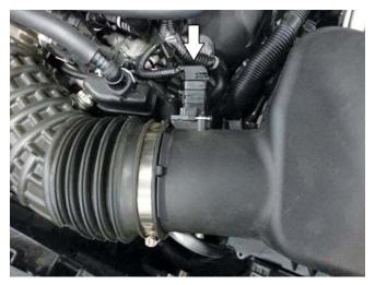
2. Loosen the hose clamp holding the air box lid to the intake tube.
