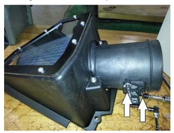
Install the air box assembly into the vehicle and fasten it using the 5 takeout screws. Torque to 3 Nm.
