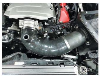
6. Using the constant tension clamps (CT-28) and (CT-32), install the sound tube and the PCV line into the clean air tube. The larger diameter clamp is for the sound tube.
