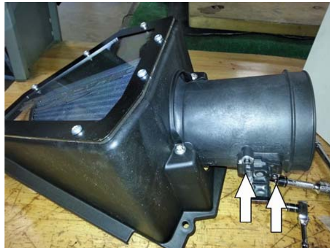
8. Install the air box assembly (2116-9A612) into the vehicle and fasten it using the five (5) takeoff screws. Torque to 3 Nm.
