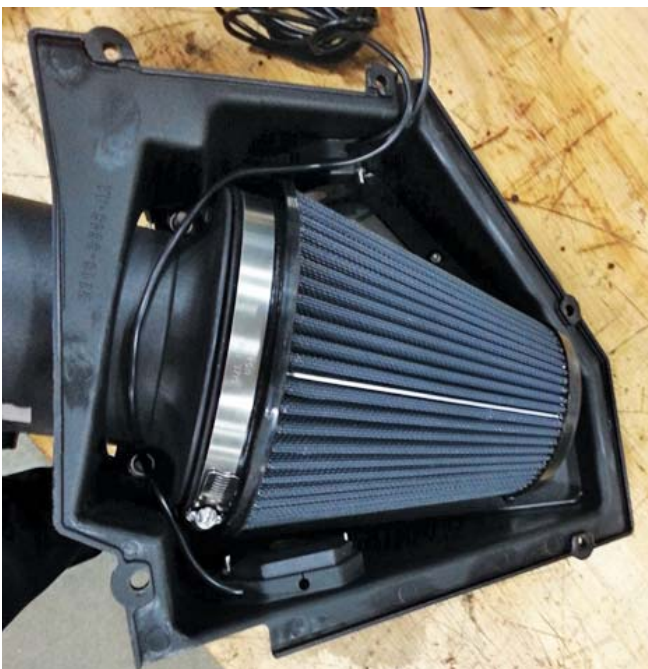
6. Install the air filter (997-484-BLK) with the metal tab pointing downwards. Tighten the clamp to 3 Nm.
