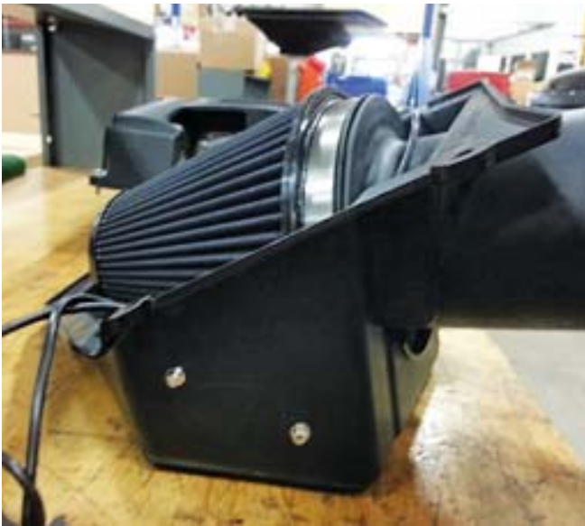
5. Run the wires out of the air box as shown.
