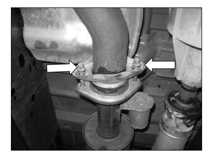
2. Loosen the clamps, which secure the intermediate pipe and resonator to the muffler and tail pipes.
