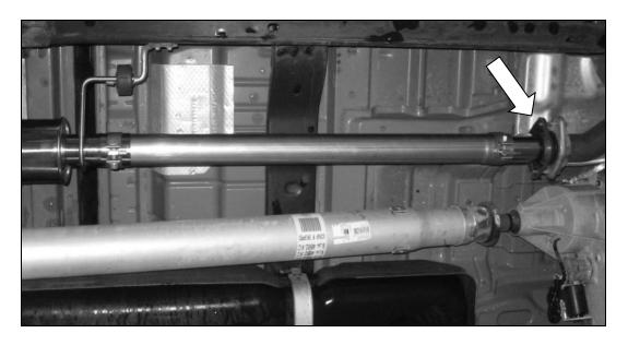
10. Install one (1) 3.0" clamp (R12060012) onto the exhaust tip and slide the tip (SLP1111-5230TIP) onto the end of the rear pipe assembly (1113SE-5C262). Position the tip so that the end is flush with the edge of the bedside, and the SLP Logo is facing up.
