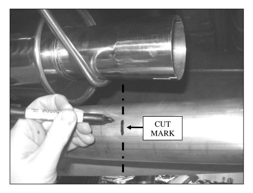
6. Remove the intermediate pipe from the catalyst adapter flange and cut the intermediate pipe at the marked length to fit your wheelbase. Make sure to double check your measurement prior to cutting the material. Remove all sharp edges after cutting.
