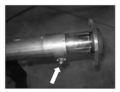
8. Insert one (1) 3" clamp (R12060012) over the end of the intermediate pipe and insert the intermediate pipe into the muffler. Position the clamp on the pipe joint and loosely secure.
