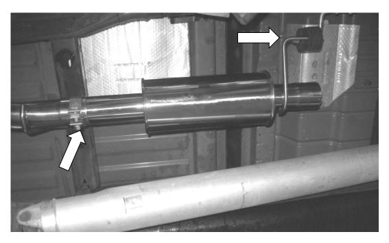
4. Position the intermediate pipe (1111-5246) into the catalyst adapter flange.
