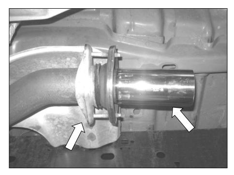
2. Position the new muffler outlet axle pipe (1111-5C262) into position and install the steel hanger brackets into the factory rubber hangers. Orient the pipe such that the flared end faces forward in vehicle.
