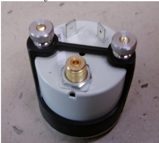
Figure 2: Cutting and deburring of the studs with the gauge locking mount installed
