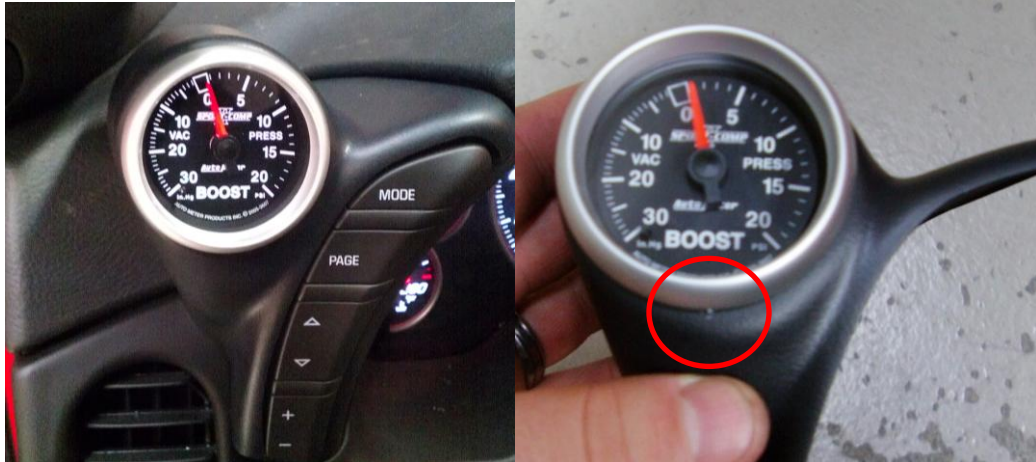
Figures 3 and 4: Mark the gauge pod for correct gauge orientation
