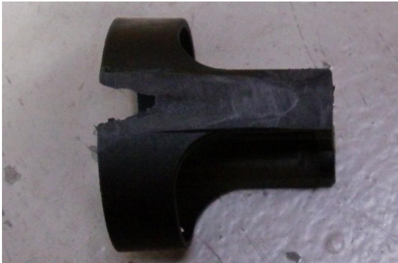
Figure 1: Bulges and back corners ground down on gauge locking mount
