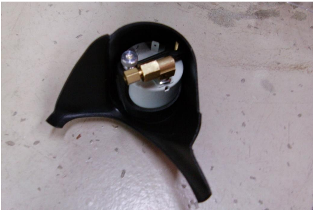
Figure 5: Gauge installed properly into pod
