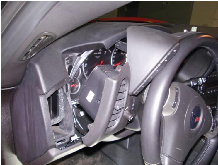
Figure 8: Removal of gauge cluster trim
