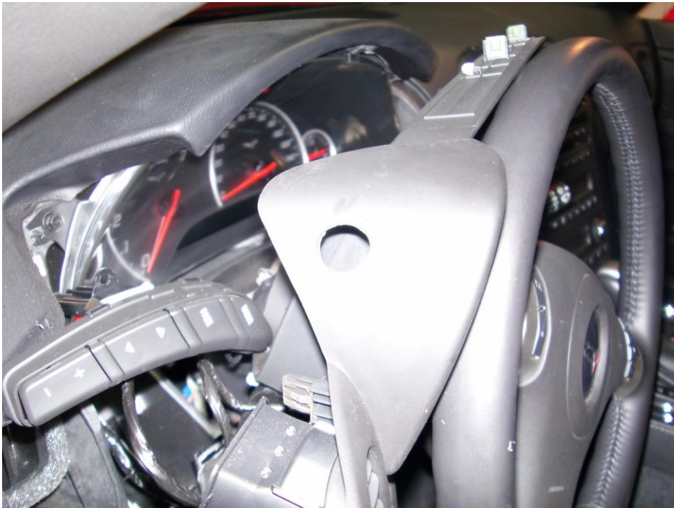
Figure 9: Drilling of the gauge cluster for compression fitting clearance
