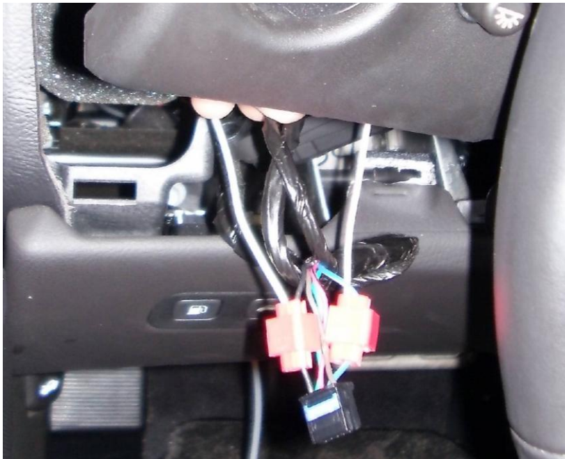
Figure 11. Use the provided wire taps to create power and ground wires for the gauge
