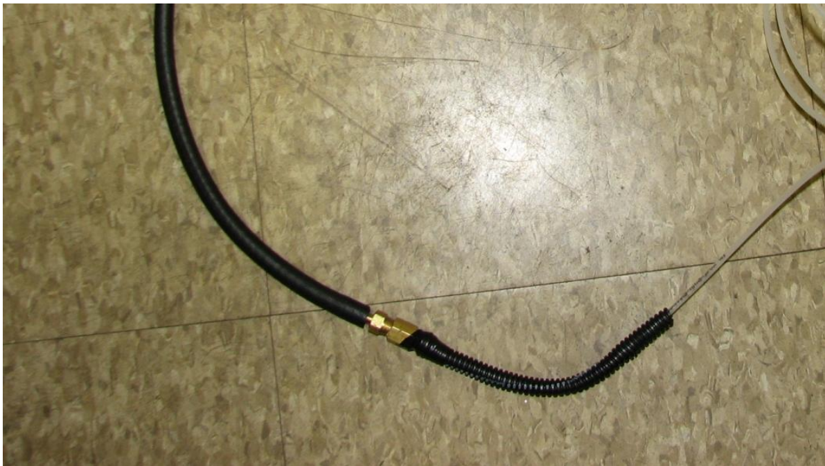
Figure 17: Vacuum/Boost tubing with fittings installed (removed from vehicle for clarity)
