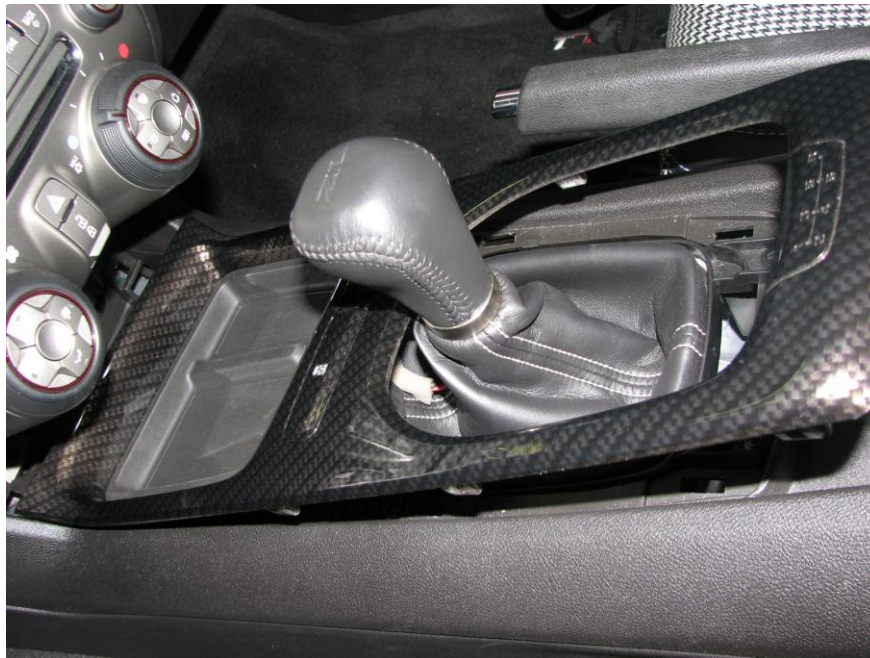
Figure 4: Removal of center console trim
