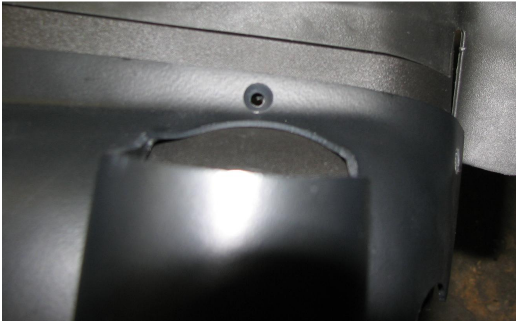
Figure 20: Drill a hole in the gauge pod at the peak of the curve as shown
