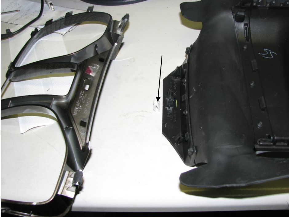
Figure 3: Separate the shroud from the gauge trim. Note the small white clip needs to be removed first
