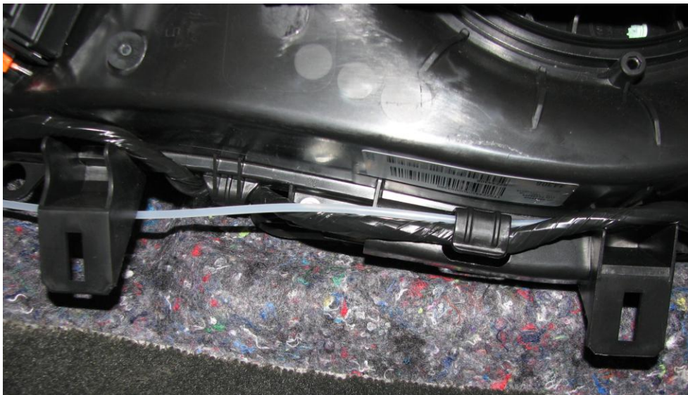
Figure 16: Tuck the vacuum line in the factory clips
