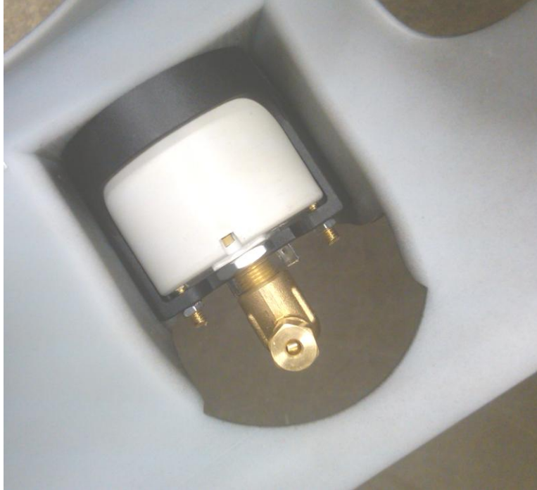
Figure 23: Snug the nuts on the gauge pod mount as shown above
