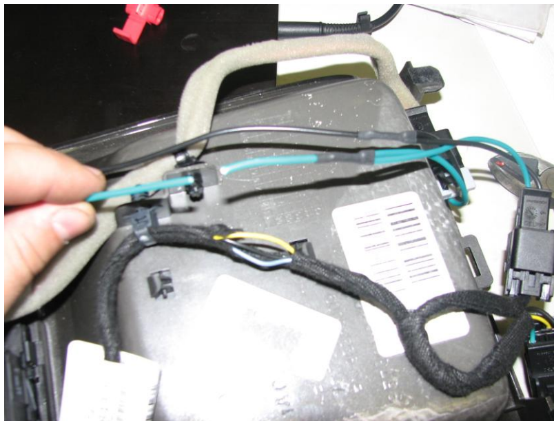
Figure 6a: Cutting of the SLP wire harness after the y-splice and exposing the yellow wire
