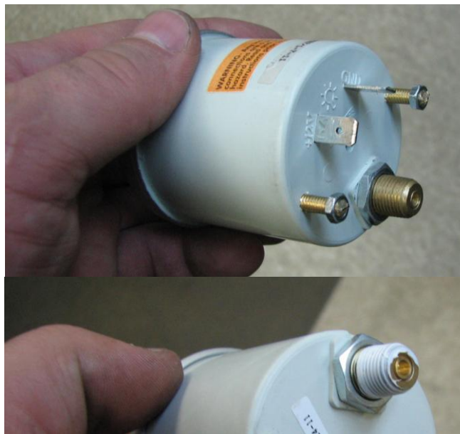
Figure 17: Wrap Teflon tape on vacuum feed on gauge/cut posts
