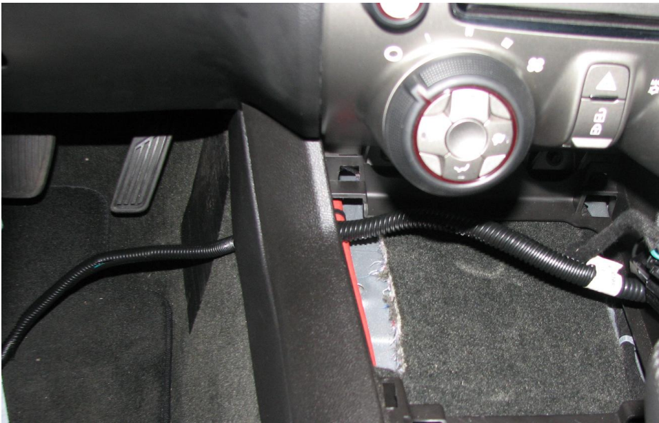
Figure 7: Snake the wire harness down in-between the plastic trim
