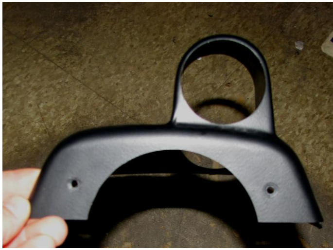
Figure 19: First two holes drilled using template
