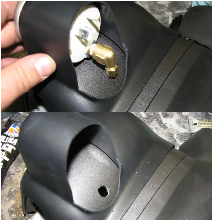
Figure 22: Before and after drilling the \frac{3}{4} " hole
