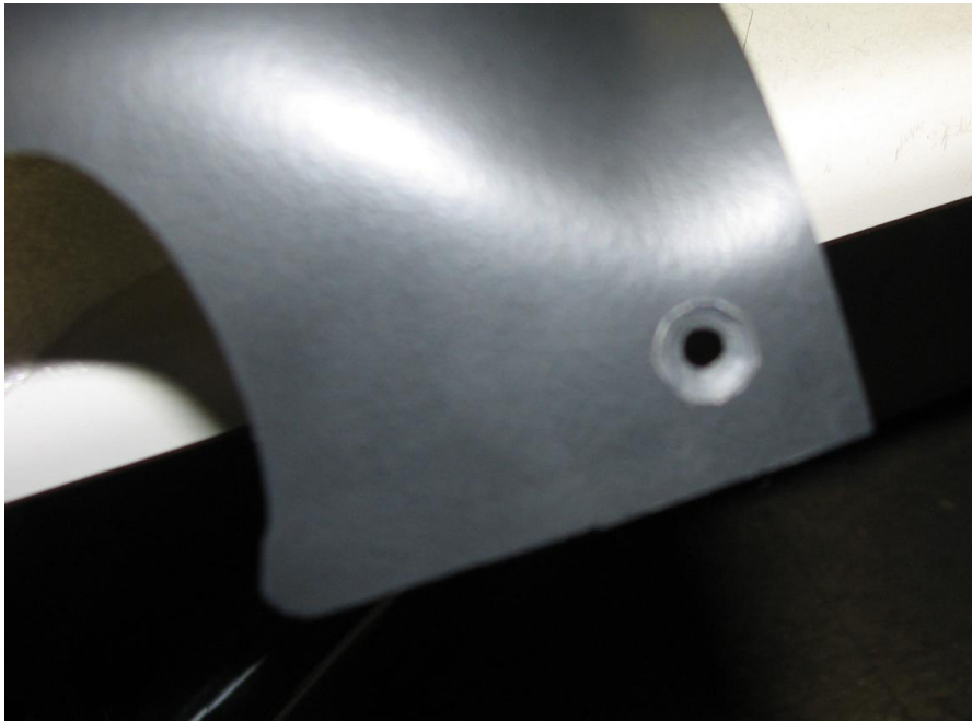
Figure 21: Drill holes \frac{1}{2} inch from back and bottom edge at back of gauge pod
