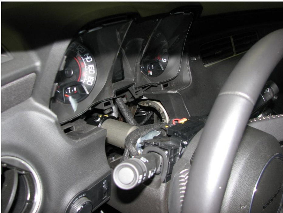
Figure 2: Removal of top shroud and gauge cluster trim
