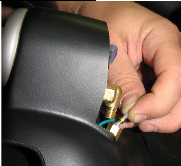
Figure 25: Fastening the vacuum line and flag terminals to the gauge
