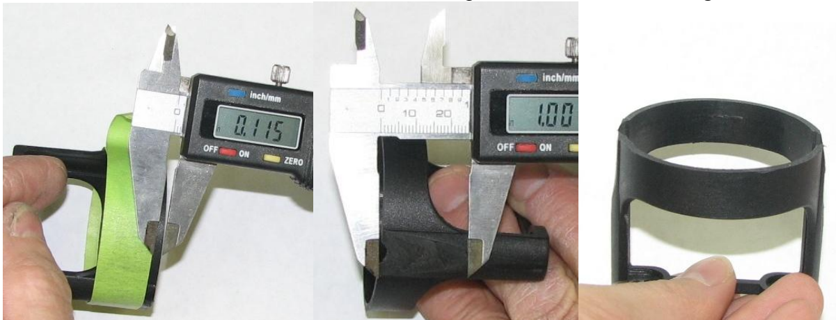
Figure 18a: cut .110-.125 away Figure 18b: Grind away to 1” Figure 18c: Final
