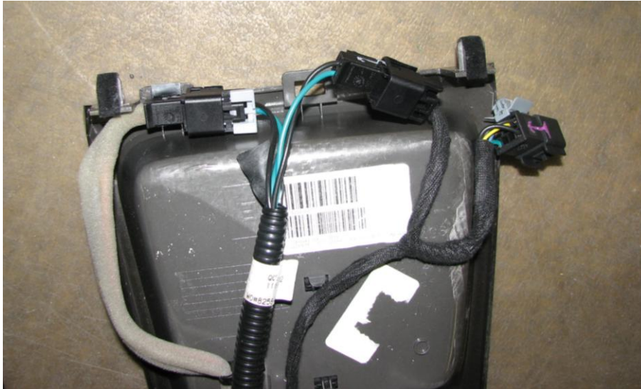
Figure 5: Installation of the SLP wire harness
