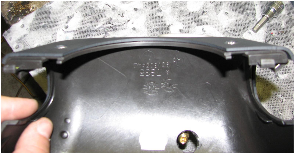
Figure 24: Front edge of gauge pod snug against shroud
