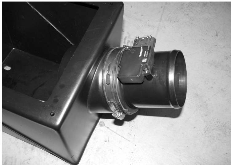
MAF and airbox adaptor placed onto airbox
