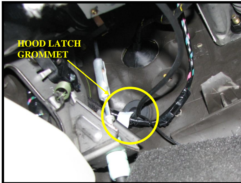
Photo 4: Hood Latch Grommet with Switch Wiring Routed Through
