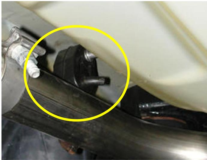
**Figure 6: Stock rubber isolater**
