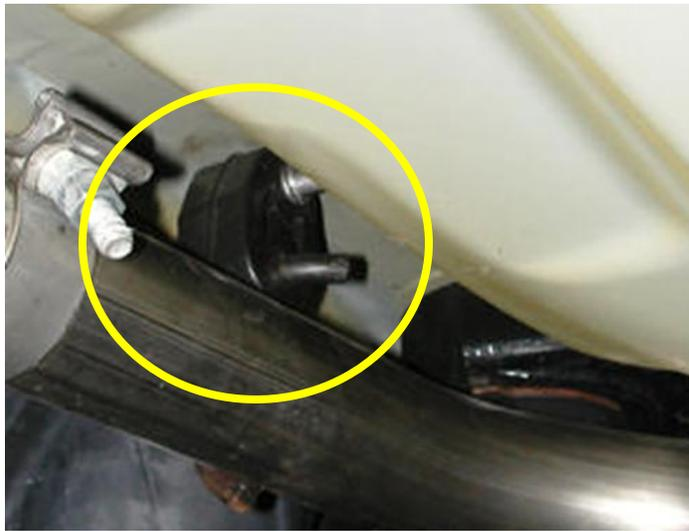
**Figure 6: Stock rubber isolater**
