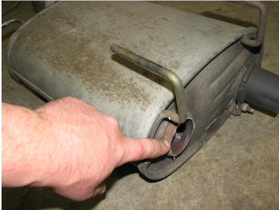
**Figure 1: Cut off factory mufflers here**
