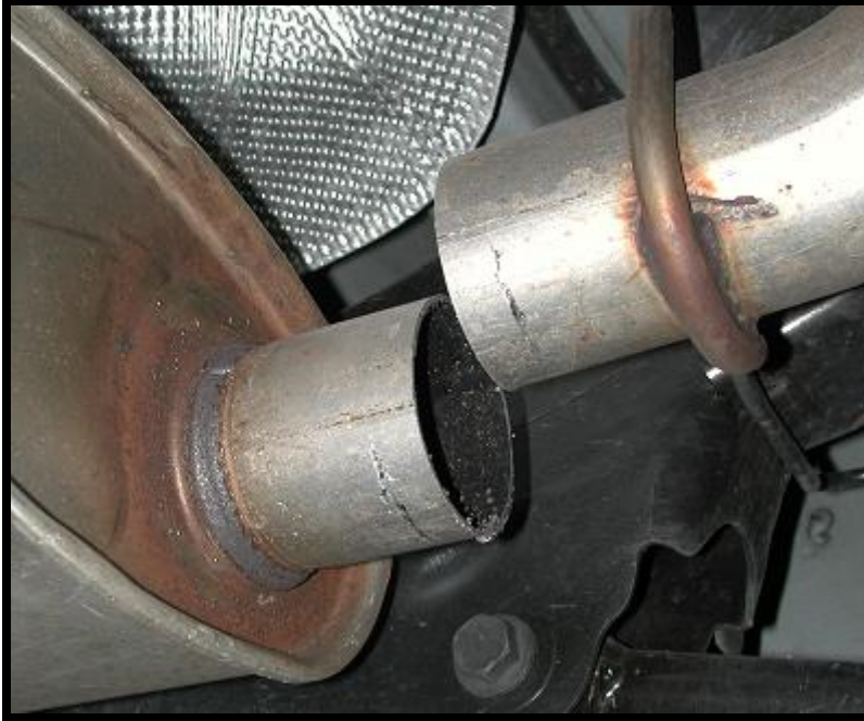
Photo 1: Muffler Cut Location
