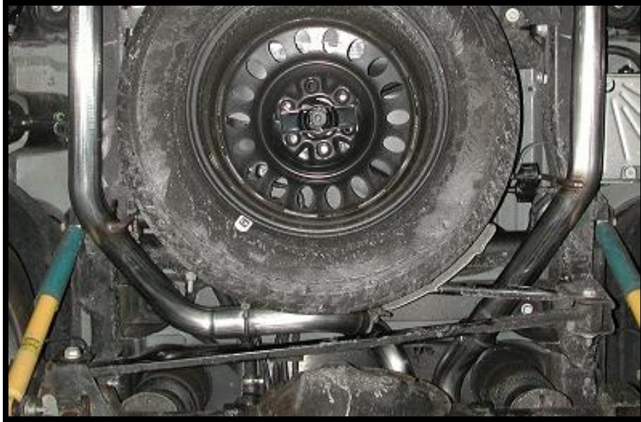
Photo 10: Tailpipes Attached to Connecting Pipes
