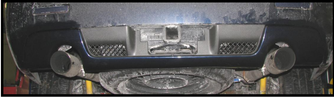
Photo 6: Valance Install Complete
