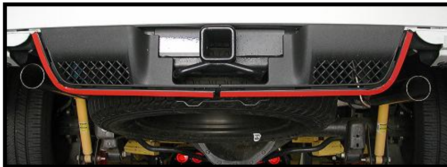
Photo 4: Adhesive Tape on Trailer Hitch Valance
