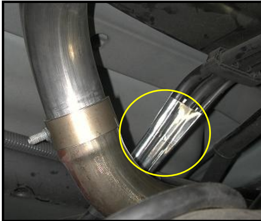
Photo 11: Fuel Lines Wrapped with Heat Tape
