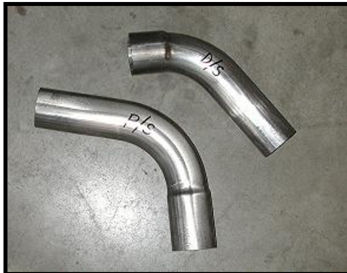
Photo 9: Over-Axle to Tailpipe Connecting Pipes
