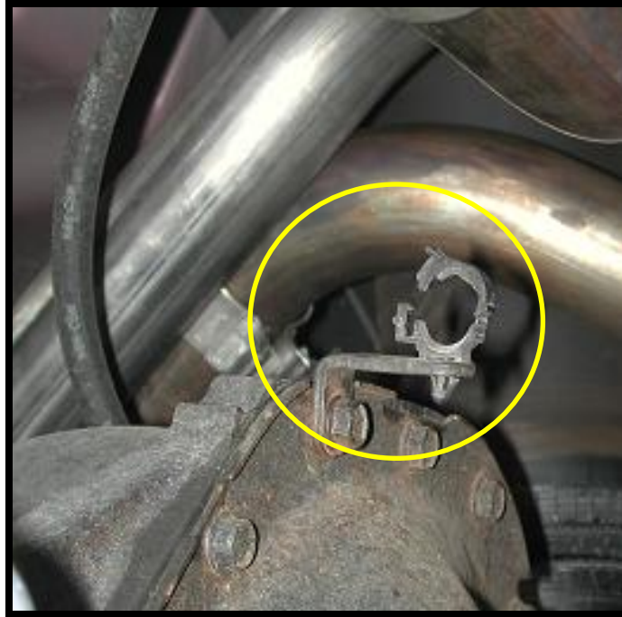
Photo 12: Vent Hose and Bracket
