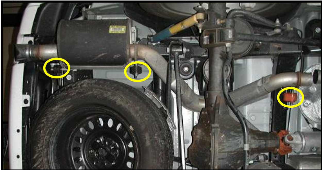
Photo 2: Stock Resonator Pipe Hanger Locations
