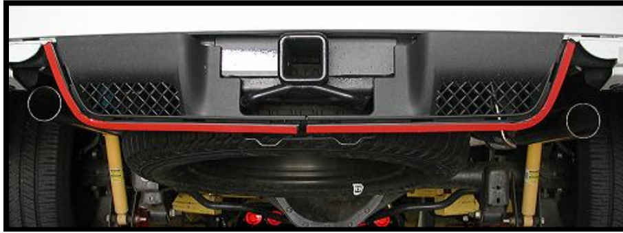
Figure 3: Adhesive Tape on Trailer Hitch Valance
