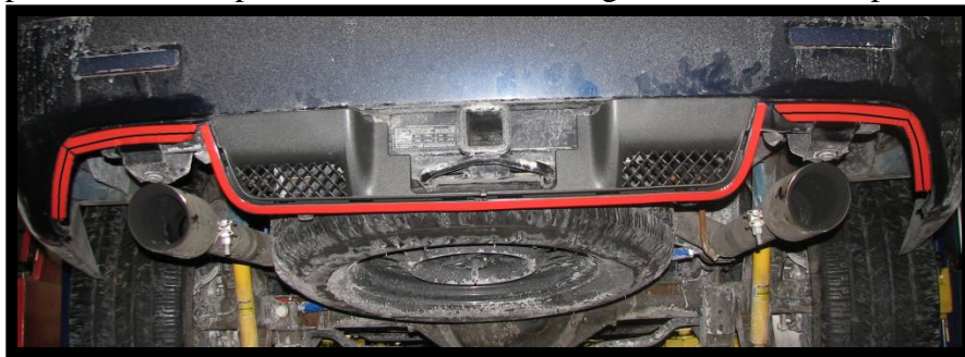
Figure 4: Adhesive Tape on Rear of Vehicle
