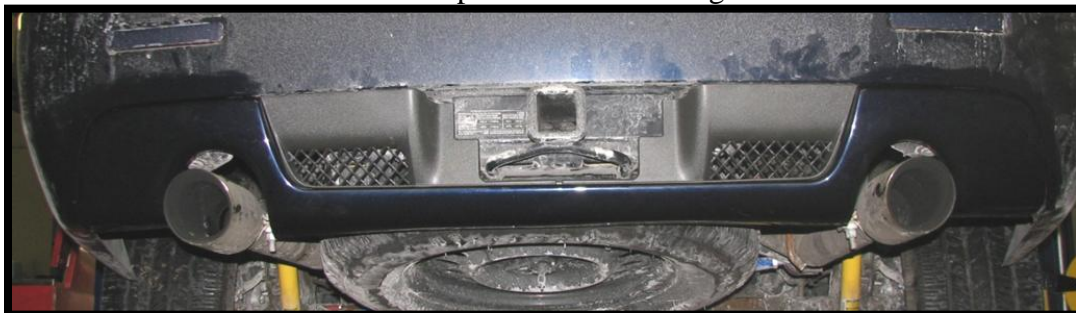
Figure 5: Valance Install Complete
